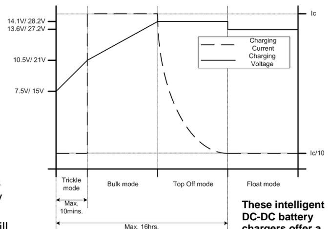
These intelligent DC-DC battery chargers offer a comprehensive 4 stage charging programme as well as protection against battery source drainage. A fifth terminal is also available to allow the unit to be installed as a float-mode charger if required as an alternative.
